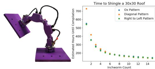
**Simulation.** We modeled the physics of inchworms, shingles, and a roof in Gazebo using an open-source magnet plugin. Our system can simulate any roof and swarm configuration. To quickly test and evaluate different swarm behaviors, we also developed a lightweight simulator to model a swarm of robots shingling a roof. This simulator allowed us to rapidly test novel decentralized shingling algorithms, and evaluate the performance of differently sized swarms.
